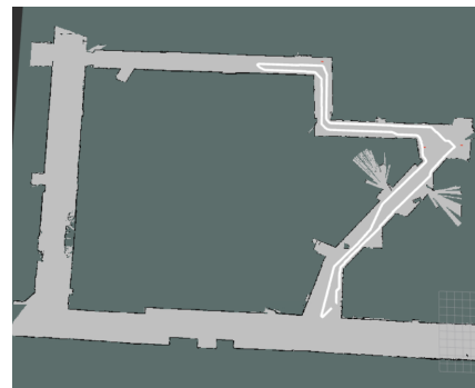
Figure 7: More optimal path planned with a U turn in the middle.
